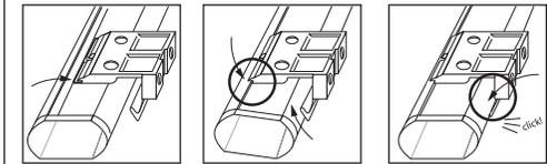
For style 'B' [see illustration]: Lift the Head Rail into position such that the front edge of the bracket is under the inner front edge of the head rail, and then push the head rail upward until the flexible tab at the bottom of each bracket snaps onto the back of the head rail. Check carefully to assure that each bracket is properly secured.
