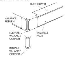
Round corners come in 3 pieces. Attach the rounded corner pieces onto the main valance, then attach return to the corner piece.
