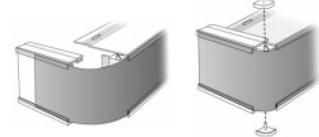
Insert the plastic top and bottom corners and push down to secure.
