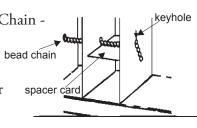
Lock the bead chain into the key holes starting with the leading vane. Four inches of chain should be between each vane. Trim excess chain one inch beyond the first and last vane.
