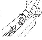
Finally, release the link by pulling upwards, otherwise function is limited.
