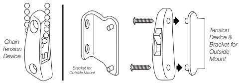
If mounting into wood, pre-drill screw holes and then install the mounting bracket using the 11/4" Phillips head screws provided.
