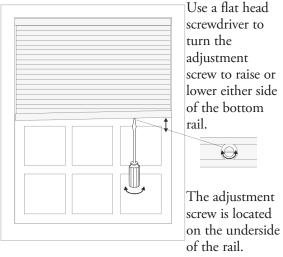
One quarter turn of the screw will move the bottom rail up or down approximately 1/4". Over-turning the adjustment screw (more than 1") can cause the cord to tangle or get pinched inside the rail. The screw should turn easily - Do Not Force.
