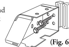
For inside mount applications there must be a minimum of 1/4" between the back of the headrail and any obstruction.
