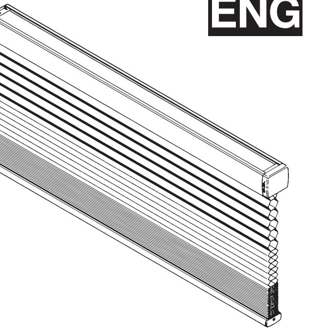
Identify the head of the motor housing on the right side of the shade (see drawing) - Press the PROGRAM button until the shade oscillates (the shade will oscillate - a quick back and forth movement of the shade) Press the UP button on the remote (see drawing) - the shade will oscillate again - the motor and transmitter are now mated.
