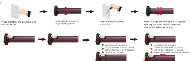
press the PROG button for 1s motor head will flash red 1 time then release your hand
